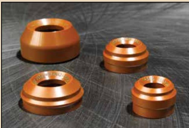
Meldin® **7001** is used as a thermal insulator in hot runner nozzles used for injection molding thermoplastics such as PET bottle preforms. Designed and manufactured especially for molding thermoplastics of all kinds, the nozzle tip insulator serves two purposes: thermal insulation of the molten plastic to prevent freeze-off of the plastic while awaiting injection inside the hot runner system, and allowing easy color transfer between production batches, reducing downtime of the tool.
