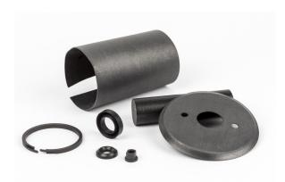
Rulon® 123 is a glossy black non-abrasive compound for softer mating surfaces, such as stainless steel. This material has excellent chemical resistance and is FDA and USDA compliant. It is less expensive than Rulon® J, but is slightly less flexible and higher in wear.
