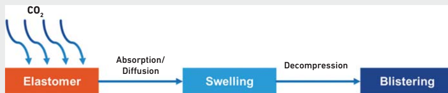
Fig. 1: Schematic showing the events leading to blistering of polymers when depressurized after being exposed to a high-pressure CO 2 [3]
