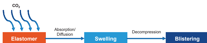
Figure 1: Schematic showing the events leading to blistering of polymers when depressurised after being exposed to a high-pressure CO 2 (Source: TWI, "Selection of materials for high pressure CO 2 transport", paper presented at Third International Forum on the Transportation of CO 2 by Pipeline, Newcastle, June 2012)
